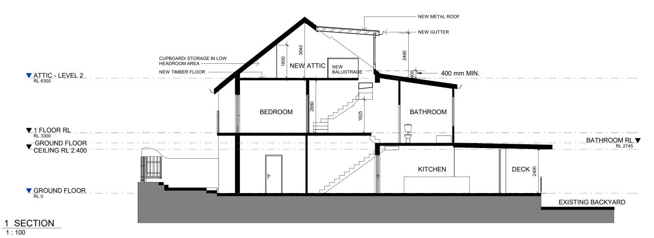
NEW METAL ROOF THE APEX OF THE GABLE OR TOP OF THE DORMER ROOF IS TO BE AT LEAST 200MM BELOW THE RIDGE LINE OF THE MAIN ROOF — NEW TIMBER WINDOW No 63 NEW DORMER **NEW ATTIC** - CUPBOARD/ STORAGE IN LOW HEADROOM AREA ATTIC - LEVEL 2 400 mm MIN FRONT WALL BATHROOM **BEDROOM** ▼1 FLOOR RL RL 3300 ▼ GROUND FLOOR CEILING RL 2.400 DECK KITCHEN LIVING ROOM ▼ GROUND FLOOR EXISTING BACKYARD 2 SECTION
